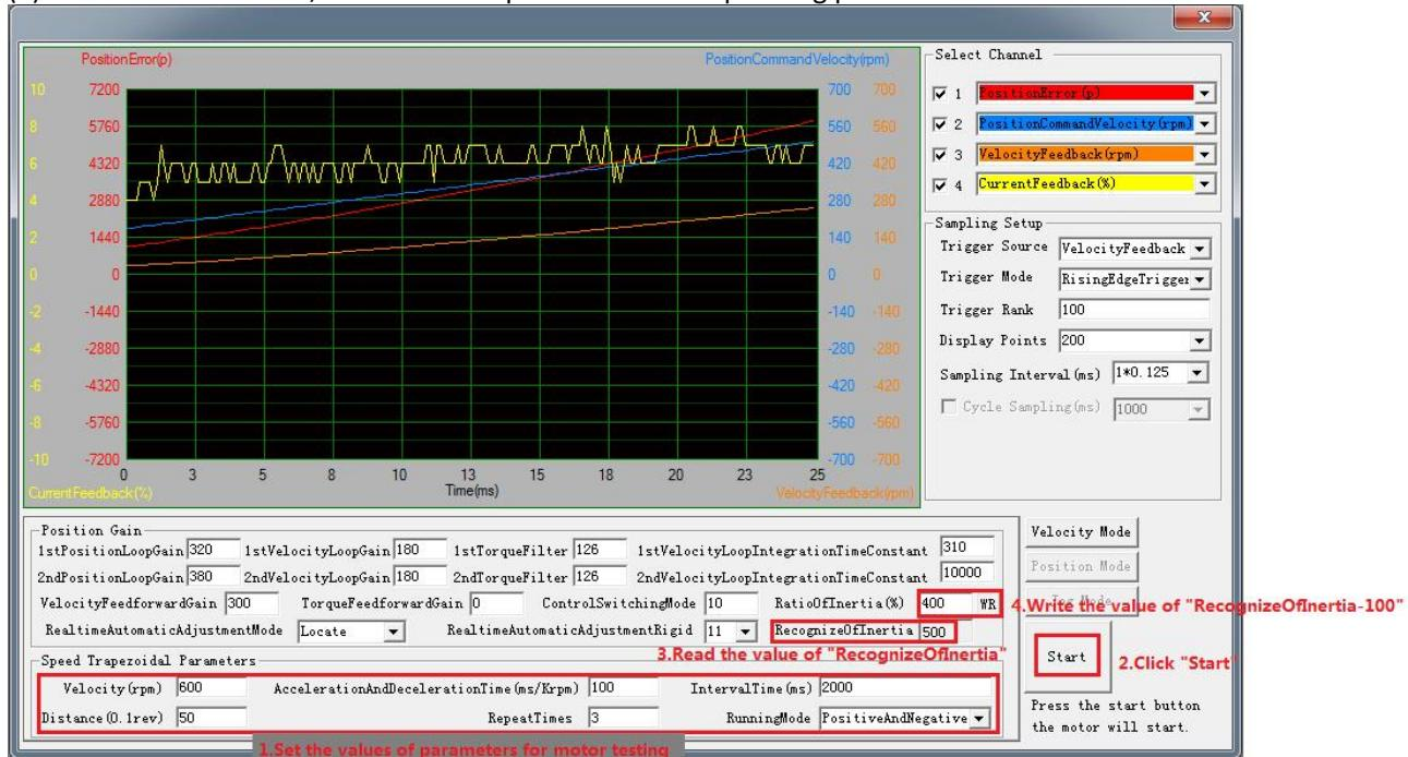
The value of the load inertia ratio obtained from the above steps can satisfy most applications, but for some cases where the load inertia is very high, the value of Pr0.04 can be increased to more than 1000.
