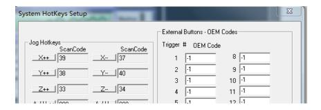
Set the hotkeys of X. Y. Z axis as this diagram, then you can control the motors by this hotkeys on the keyboar.
