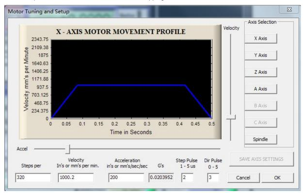
Steps per is means how many steps it need for moving 1 mm. The seting of Y Z A axis is similar to X, and please save the settings after all. Please set Step Pulse at least 5 us for driver M542T and M860H.
