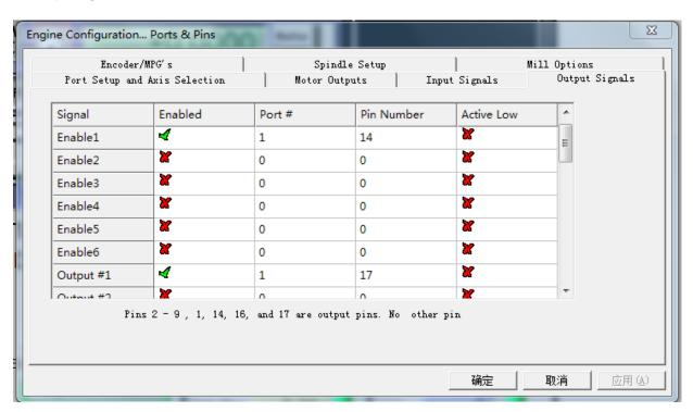
Enable1: stepper motor enable setting. --p14 Output #1: spindle relay switch setting. --P17
