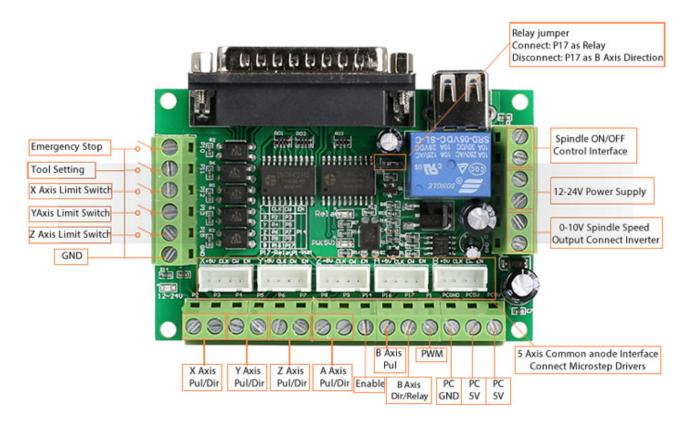
Note: all the seting below is for common anode connection between this interface board and the stepping motor drivers.
