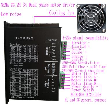
32 bit DSP digital step motor driver
